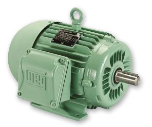
WQuattro is a hybrid motor with squirrel cage rotor fitted with high energy permanent magnets making it suitable for direct on line start.
