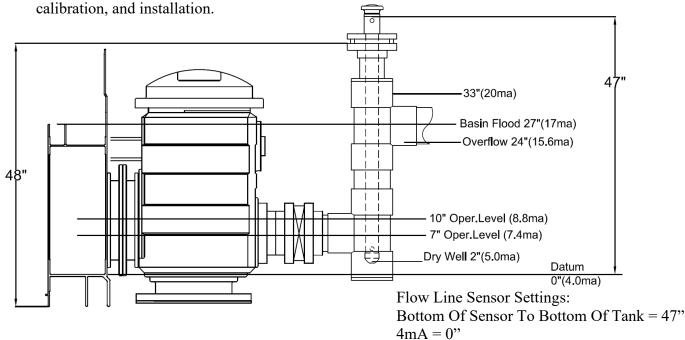
Figure 18B – Sump Detail With Ultrasonic Liquid Level Sensor
