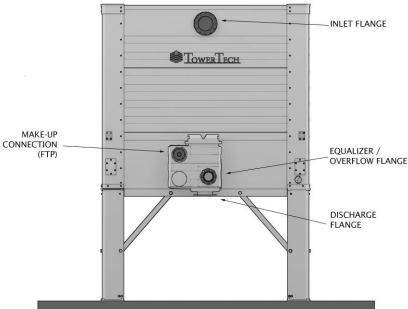
Figure 36 – Standard Piping Connections
