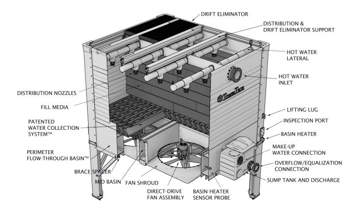
Figure 1 - TTXR 3-D Cut-Away View
