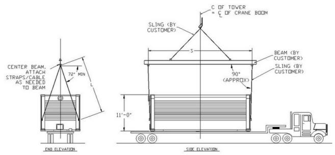
Figure 34 - Tower Lifting Procedure
