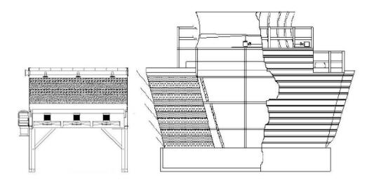
Figure 2 - TTXR versus Conventional Induced-Draft Cross-Flow Tower
