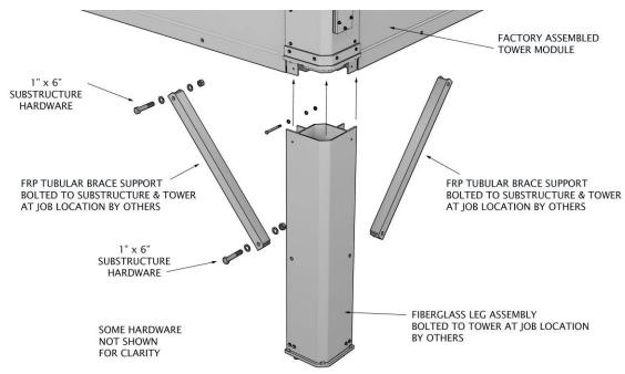
Figure 14 – Tower Sub-Structure
