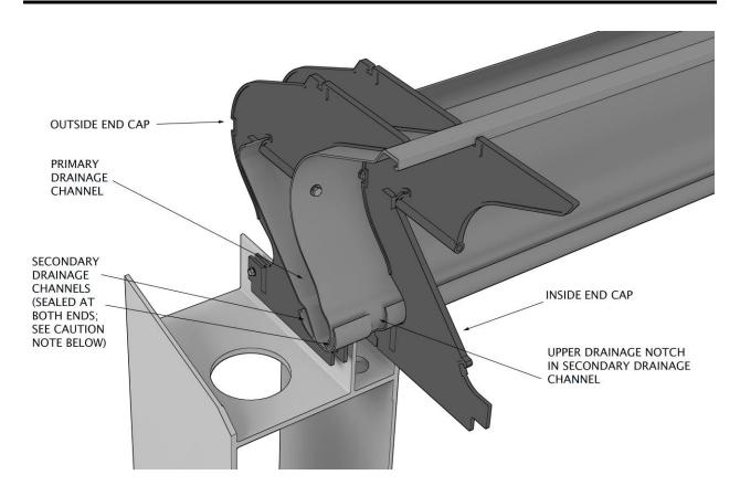
Figure 59 - Close-Up View: Water Collection System
