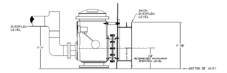
Figure 45 – Sump Level Control Detail
