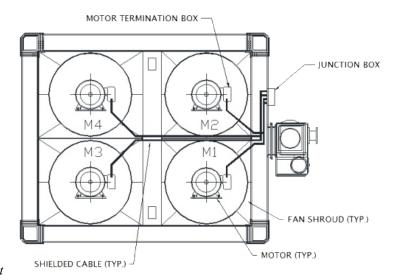
Figure 12 – Typical Wiring Layout
