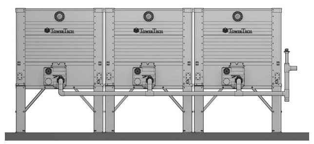
Note: Keep all vents clear and open. Stand pipes must be heat traced and insulated in cold climates.
