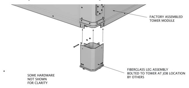
Figure 30 – Installation Detail for 1' Sub-Structure
