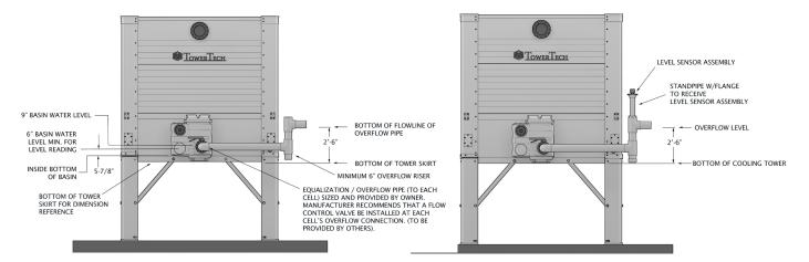
Figure 39A – Typical Overflow/Equalization Pipe
