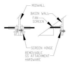
Figure 54 – Close-Up: Fan Guard Hardware
