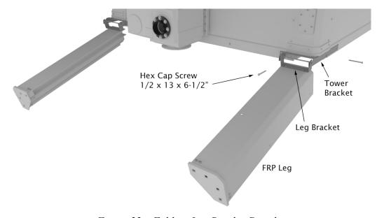
Figure 22 – Folding Leg Bracket Detail
