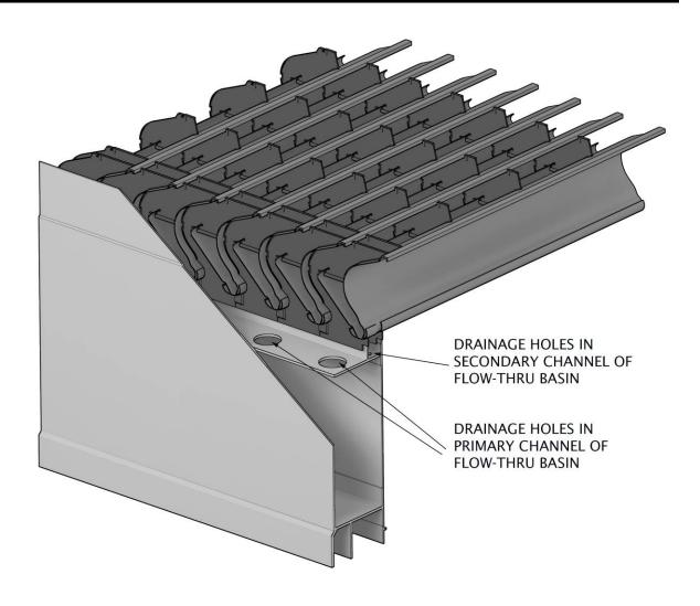
Figure 60 - Flow-Thru Basin Drainage (Perimeter Basin Wall)
