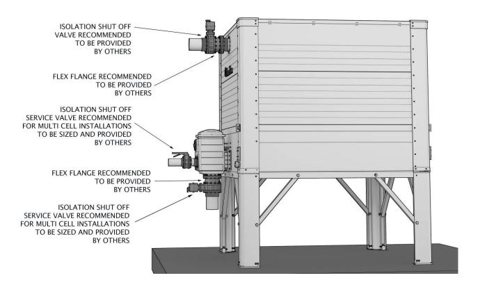
Figure 37 - Connection Flexible Flanges & Flow Control Valves
