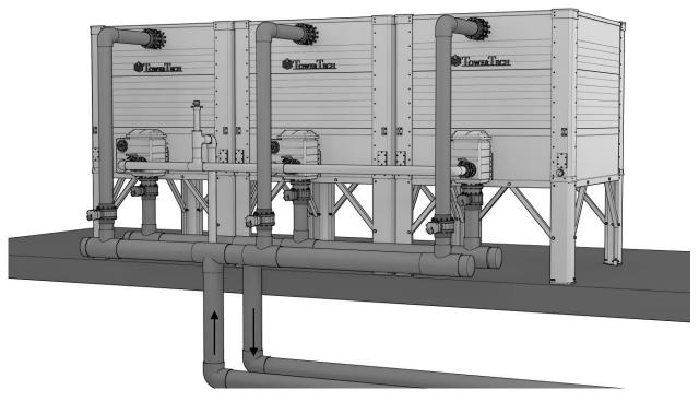
Figure 21 – Multi-Tower Layout and Piping Recommendations
