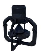
The innovative nozzle design is shaped to provide a square spray pattern, thereby uniformly wetting the entire fill media. This improves tower performance and reduces the likelihood of scaling due to the occurrence of dry regions
